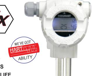
Indumart TTS360 Series of Smart Temperature Transmitters are two-wire microprocessor-based instruments, which can sense temperature via their Pt100 or type "K" thermocouple, and indicate the value of temperature on the wide LCD display, and generate a 4-20 mA output signal directly or inversely proportional to the temperature input. transmitter's output is fitted with a radio-noise filter and other elements protecting against ESD.
